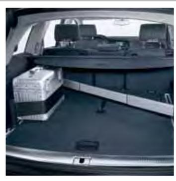
Load-securing set with rails
