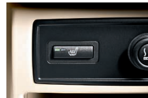
□ 496 Seat heating, rear: same as 494 (seat heating, front) but with heating in two stages, or three stages in conjunction with 4NB (automatic air conditioning with four-zone control).
