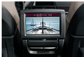
□ 6FF DVD system, rear: offers an independently controllable DVD player with a fold-down 8" screen. The system can be operated by wireless remote control, has sockets for two headphones and a video source, and is compatible with infra-red headphones (included, for two passengers) 1 . Viewing of TV is also possible in the rear, both stationary and on the move, in conjunction with 601, TV function.
