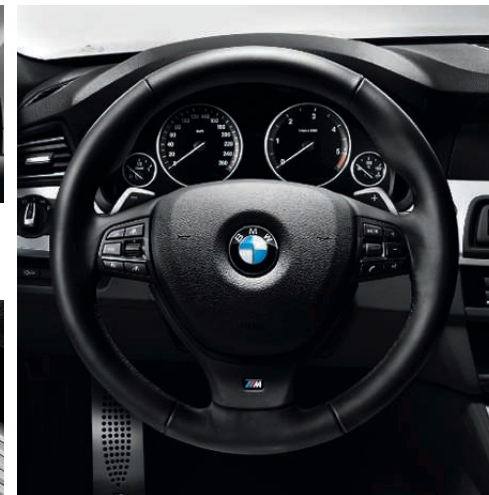
■ M Sport leather steering wheel features special thumb rests and a thicker rim for extra grip. (Steering wheel paddles shown are included with the optional sport automatic transmission. M footplate is not available for UK specification.)
