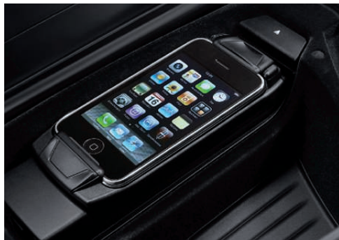
Snap-in adapter with USB interface for making calls and charging the phone together with improved reception via an external aerial. In conjunction with 6NF, also available with USB interface for listening to music.
