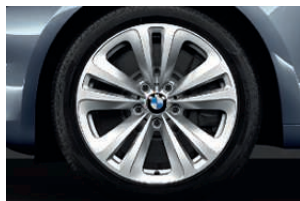
□ 2SR 18" light alloy Double-spoke style 234 8 J x 18 with 245/50 R18 run-flat tyres (standard on 535i GT, 530d GT and 535d GT).
