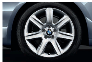
□ 2SW 19" light alloy Star-spoke style 272 with mixed tyres, 8.5 J x 19 wheels and 245/45 R19 run-flat tyres at the front, 9.5 J x 19 wheels and 275/40 R19 run-flat tyres at the rear (standard on 550i GT).
